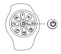
If you have used the wrong sequence to connect the remote control to the vibration plate, just switch off the plate at the main switch. After approximately 10 seconds, switch it on again and try to connect the remote control with the vibration plate again.
